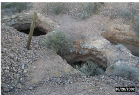
Stope openings that are 50-100 ft deep. These opening did not serve as significant wildlife habitat and were therefore backfilled.
