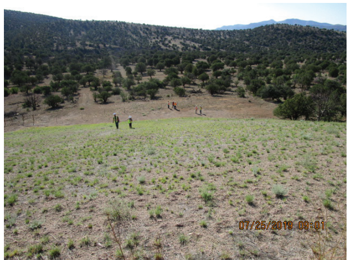
Rubio Peak test plot, testing material to be used as cover on the waste rock piles at the Chino Mine, Grant County (2019)
