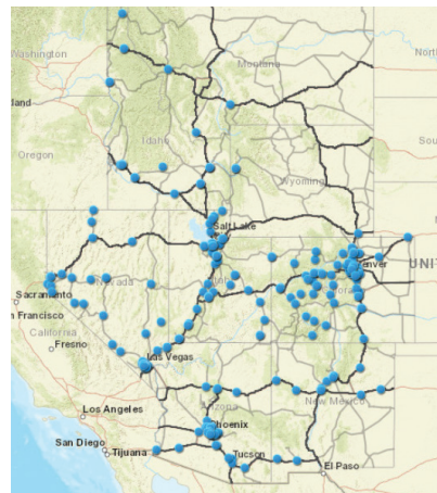
REV West Regional Planning Map highlighting existing DCFC stations and proximity to Interstate Highway corridors as of December 2020. Source: Utah Department of Transportation
