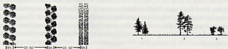
FIG. 5 A bird's-eye view (top) and a ground level view of this windbreak design shows a 6-foot space between rows and 25 to 50 feet between each set of rows. Row 1 could be juniper trees, Row 2 pine trees, and Row 3 shrubs or broadleaf trees. This windbreak design will take about the same amount of land as a traditional, four-row, normally spaced windbreak.
