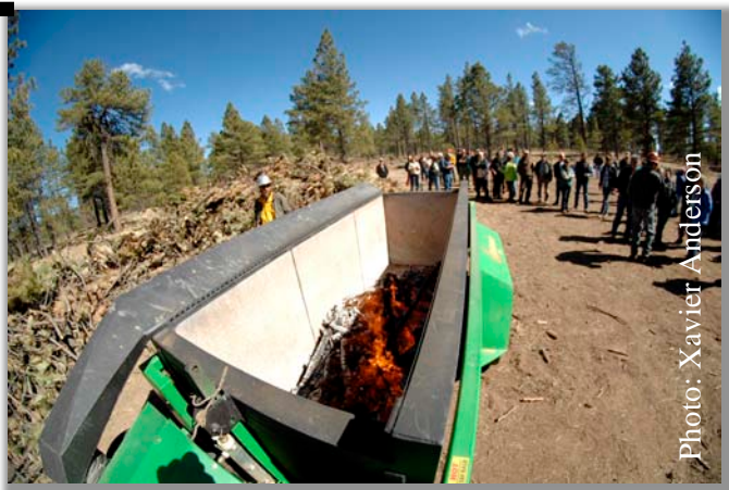
Image 2. Participants at a 2014 New Mexico Wildland Urban Interface Summit watch a demonstration of the Village's air curtain burner
